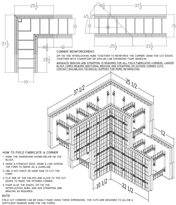
THESE DIMENSIONS DO NOT MATCH FACTORY CORNERS. CUTS SHOULD BE MADE WITH THE MOST ACCURATE SAW AVAILABLE. FIELD MITERS SHOULD BE REINFORCED WITH WOOD OR METAL STRAPPING AND BRACED ADEQUATELY. SEE THE BUILDBLOCK INSTALLATION & TECHNICAL MANUAL FOR MORE DETAIL ON STRAPPING AND BRACING.
