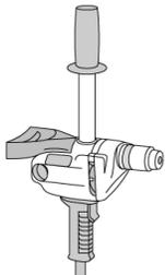
Mixing BuildCrete in easy but can be made difficult without the right mixing equipment. Smaller projects are generally batched one unit at a time and mixed in a 10-gallon bucket (available from restaurant supply companies.) Drills with plaster mixing paddles are commonly used for this purpose. A ½" (12mm) 7-amp variable speed drill with 650 rpm is commonly used for bucket batching.
