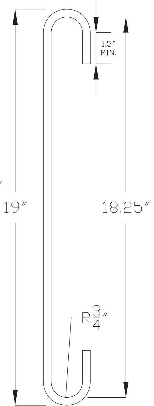
RECOMMENDED STIRRUP FOR BD-1200+8" RISER
