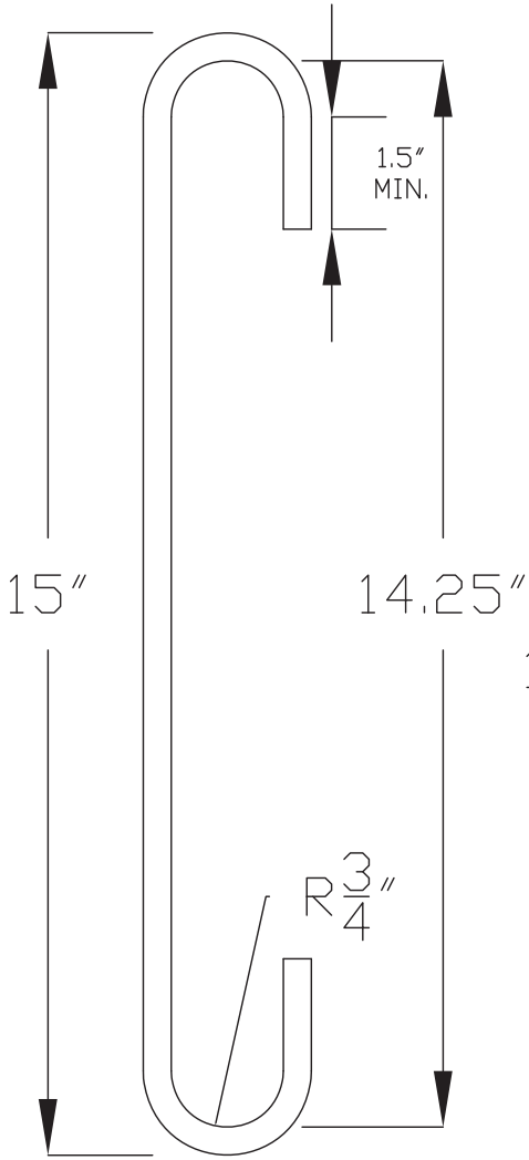
RECOMMENDED STIRRUP FOR BD-1200+4" RISER
