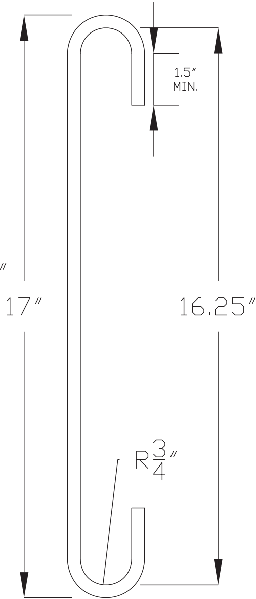
RECOMMENDED STIRRUP FOR BD-1200+6" RISER
