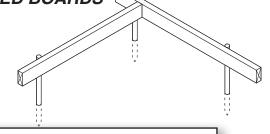
SOLIDLY ATTACH SCREED BOARDS Concrete produces downward tension in fabric. Use 3 nails or 2 screws (2-1/4") per stake.
