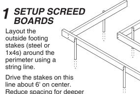
Reduce spacing for deeper footings or if the ground is less dense.
