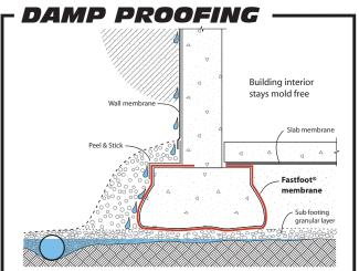
Leave screed boards & stakes in position. Pull Fastfoot® off screeds and tape two edges together on top of footing with 2" sheathing tape. Form and pour wall. After stripping (if required) run 12" width of peel & stick membrane along top of footing (covering staple holes in Fastfoot®) and up side of wall. Lap bottom edge of wall membrane over vertical peel & stick. On the inside, tape underslab membrane to interior Fastfoot®.
