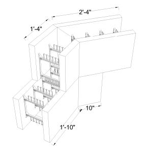
FIELD CUT CORNERS CAN BE MADE EASILY USING THESE DIMENSIONS. THE CUTS ARE DESIGNED TO ALLOW SUFFICIENT RUNNING BOND FOR THE FORMS.
