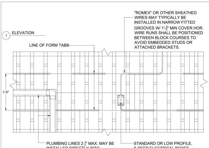
PLUMBING LINES  $2\frac{1}{2}$ " MAX. MAY BE INSTALLED DIRECTLY INTO POLYSTYRENE VOIDS POST CONCRETE POUR-PLUMBING LINES EXCEEDING  $2\frac{1}{2}$ " MAY BE INSTALLED & CAST EMBEDDED INTO CONCRETE CORE - REFER TO CODE & APPLICATIONS LIMITATIONS.
