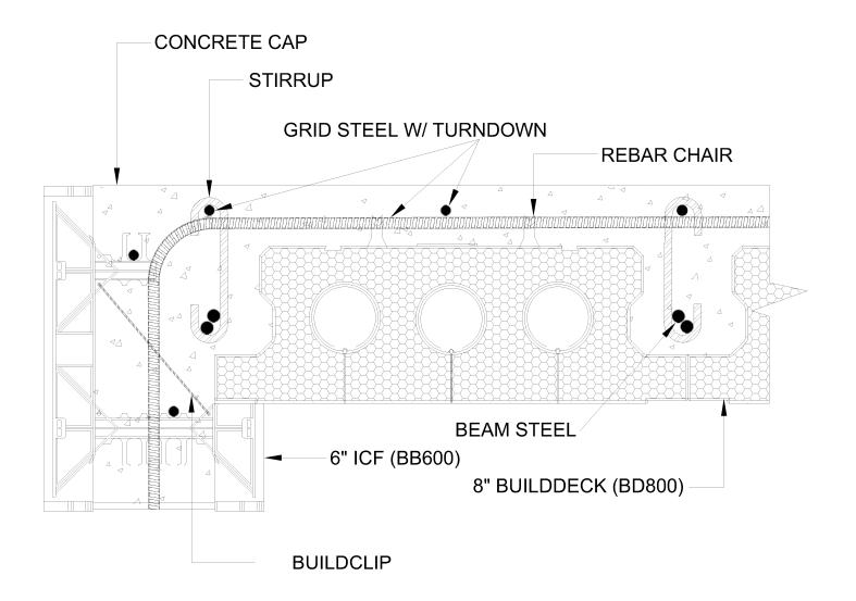
BUILDCLIP IS USED TO SUPPORT THE OUTER TOP SECTION OF A BUILDBLOCK ICF WHEN THE INNER PANEL HAS BEEN TRIMMED TO ALLOW CONNECTION TO A CONCRETE SLAB OR DECK APPLICATION. USE WITH BUILDDECK AS SHOWN.
