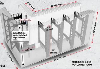
**OPEN WEB DESIGN.** Interior rebar saddles provide rebar support even when cutting half height blocks without compromising concrete flow.
